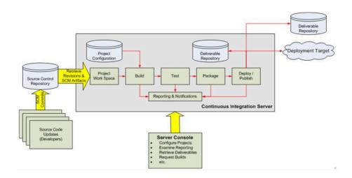
Figure 2.4: Basic Structure of CI System (Trimios, 2012)
